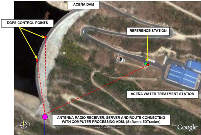
Fig. 6 DGPS spatial arrangement in La Aceña Dam
