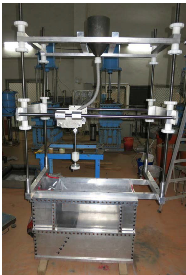
Fig. 5 Sand pluviator on the fault simulation container
