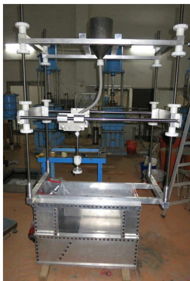
Fig. 5 Sand pluviator on the fault simulation container
