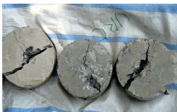
Fig. 2b Steel fibrous concrete disc specimens after failure
