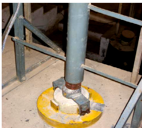
Fig. 1 Disc specimen under drop weight impact test
