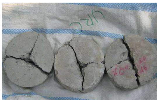
Fig. 2a Non-fibrous (silica fume) concrete disc specimens after failure
