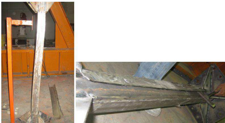
Fig. 27 Core buckling under the second mode
