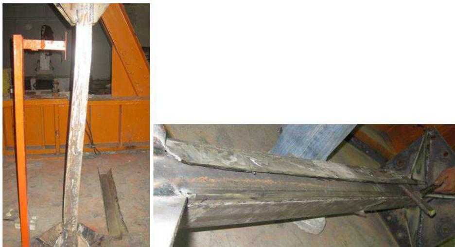
**Fig. 27** Core buckling under the second mode
