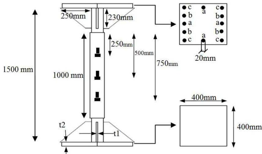
Fig. 23 details of the experimental specimens and dimensions
