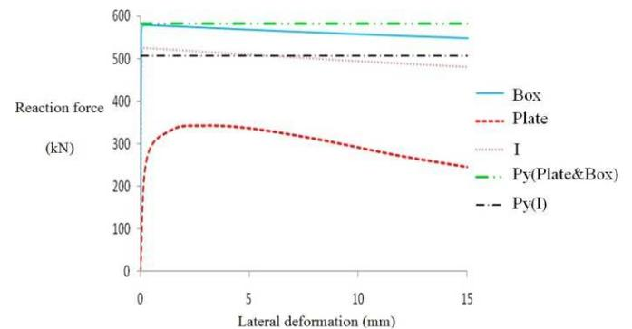
**Fig. 8** Force-displacement curves for individual core profiles
