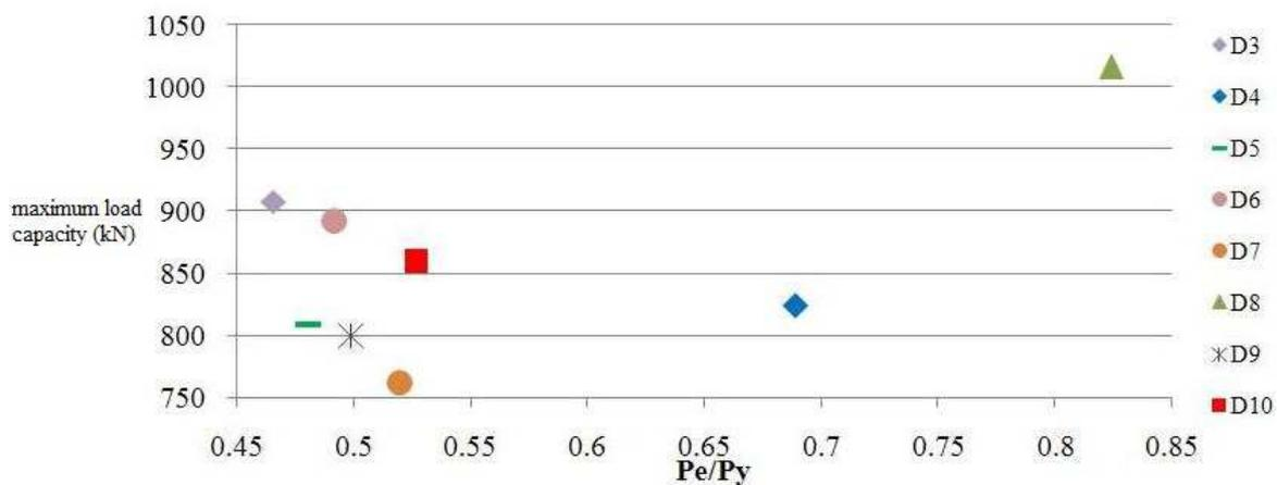
Fig. 19 maximum compressive strength of group D
