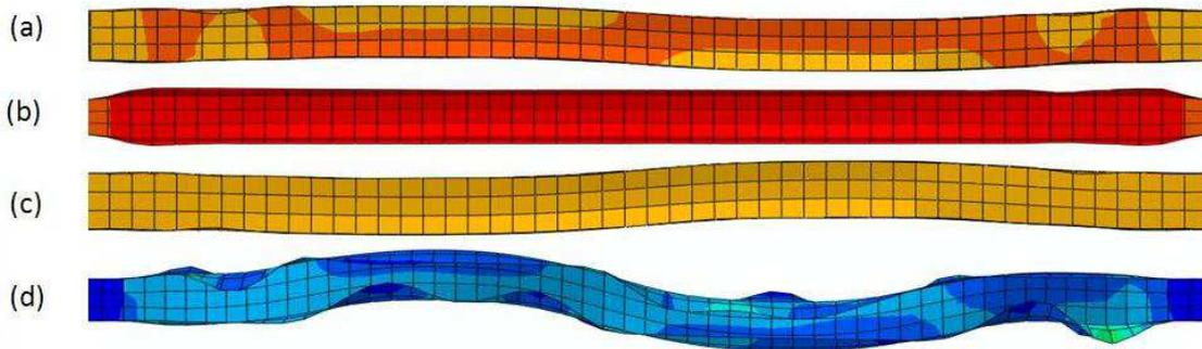
Fig. 17 lateral deformation of the cores with 15 times magnification: (a) C1, (b) C2, (c) C3, (d) C4
