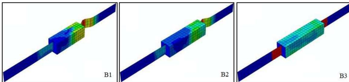
Fig. 14 Core buckling in models of group B
