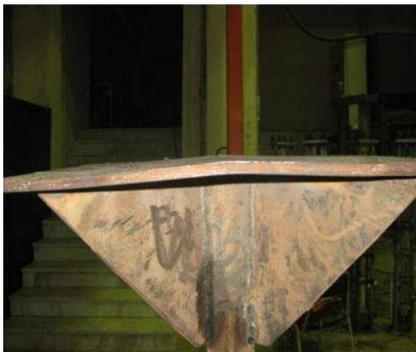
**Fig. 25** Sagged plate near the connecting bolt
