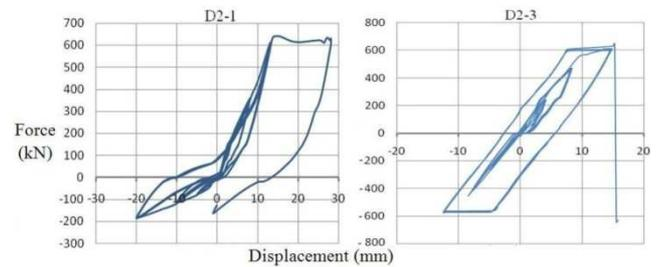
**Fig. 26** Force-displacement curve of models D2-1 and D2-3
