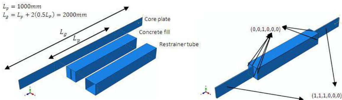
Fig. 2 overall schematic of group A of models
