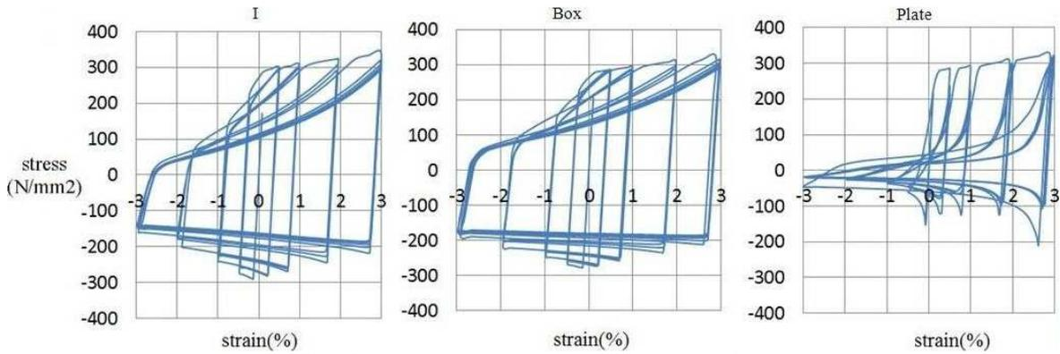
Fig. 10 Hysteretic response of individual core profiles
