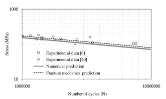
Fig. 17 Comparison of numerical predicted fatigue lives with experimental results reported in the literature
