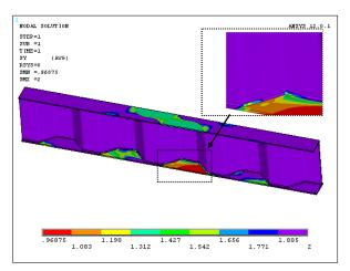
Fig. 16 Numerical safety factor contour of the corrugated web beam
