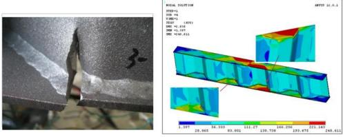
Fig. 9 Comparison of fatigue failure location with critical stress contours in modelling ( $\alpha$ =45°)
