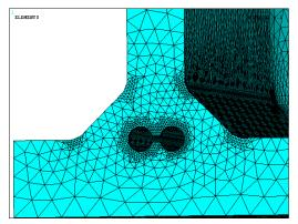
Fig. 13 Schematic of a web-to-flange welded joint in effective notch stress analysis: (a) fictitious rounding of weld toes and roots; (b) details at the intersection of longitudinal fold and inclined fold of the corrugated web; (c) local element mesh
