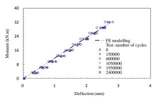
Fig. 10 Comparison of experimental and numerical moment-deflection relations ( $\alpha$ =45°)
