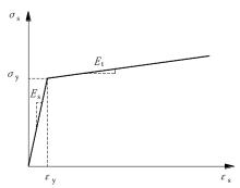
Fig. 8 Assumed stress-strain relationship for structural steel
