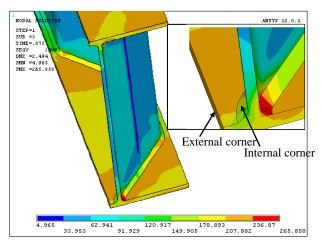
Fig. 12 Numerical stress contours at crack initiation region
