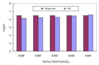
**Fig. 18** Comparison of experimental and numerical fatigue life with varying  $K_{\rm sf}$  ( $\alpha$ =45°)
