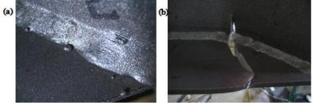
Fig. 6 Photograph of fatigue crack initiation after 1500000 cycles and failure after 3200700 cycles
