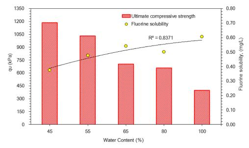
Fig. 3 Effects of ultimate strength on the solubility of fluorine for stabilized MC-clay soil at different water contents
