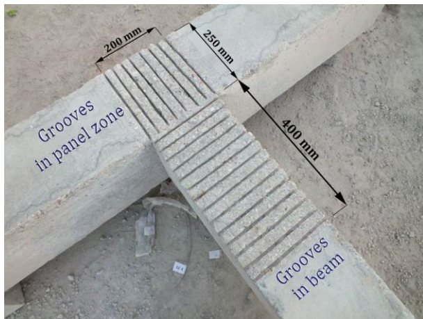
Fig. 2 Grooving pattern in specimen RW2
