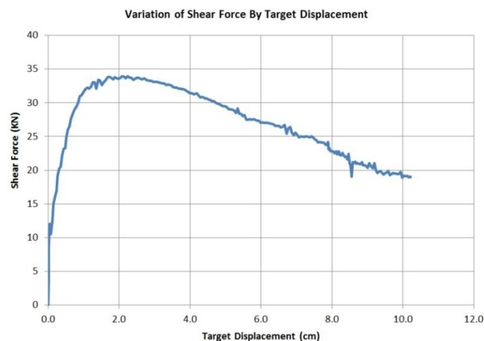
Fig. 19 Experimental behavior of RMW2 wall
