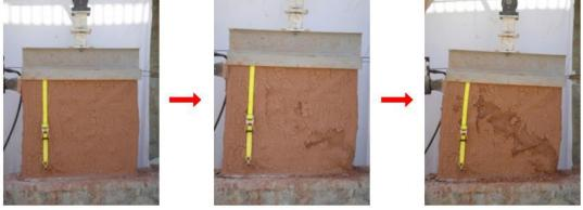
Fig. 18 Damage mechanism of RMW2 wall
