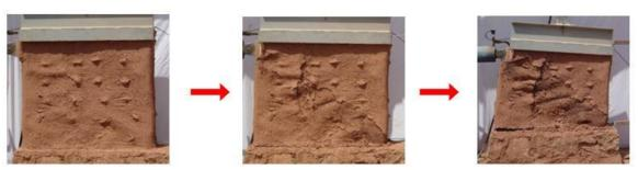
Fig. 15 Damage mechanism of RMW1 wall
