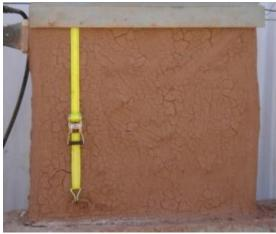
Fig. 17 Use of tarpaulin belts to prevent rocking motion mechanism
