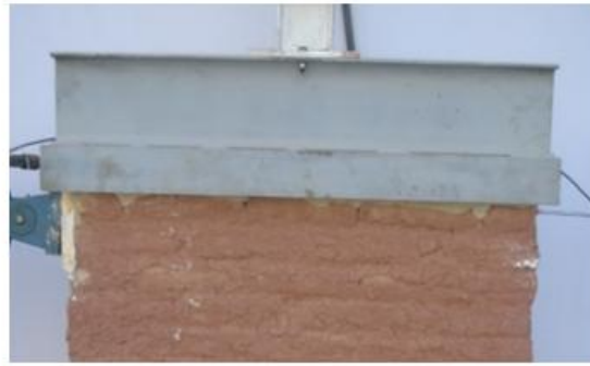
(a) (b) Fig. 6 (a) Beam section, (b) Load distribution beam
