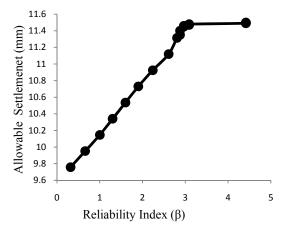
Fig. 6 Evaluation of the reliability index for different allowable settlements
