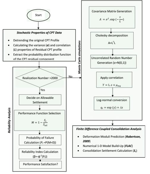
Fig. 7 Flowchart for calculation process of reliability analysis for consolidation settlement
