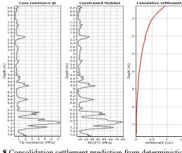
Fig. 8 Consolidation settlement prediction from deterministic analysis
